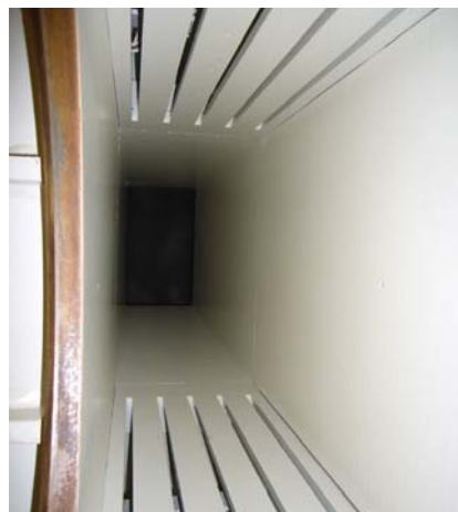
遷音速フラッタ風洞測定部 Test Section of Transonic Flutter Wind Tunnel
